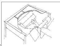
Step Number 4: Remove the stainless steel heat shield before you take out the catalytic combustor.
